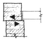
Shear cracks are sometimes due to outward pressure from vega or rafter ends. From Adobe: Practical and Technical Aspects of Adobe Conservation.
